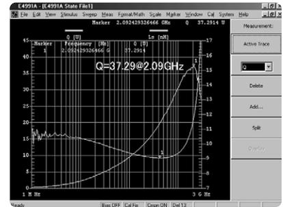
Figure 1. Ls-Q characteristics of a chip inductor
