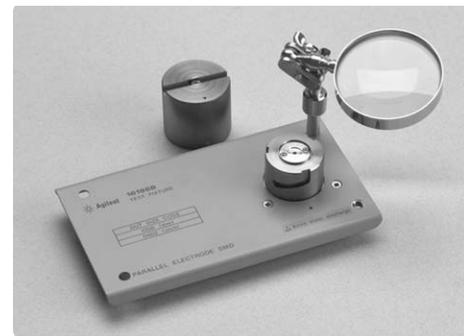
Figure 9. Agilent 16196B parallel electrode SMD test fixture
