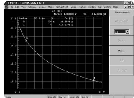
Figure 4. Varactor diode capacitance vs. DC voltage characteristics
